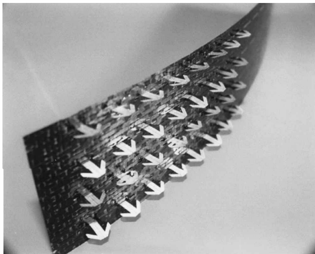
Fig. 6 TRAM subexperiment antenna module based on flexible HDI.
